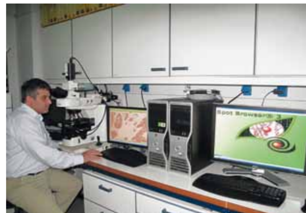
Slide Scanning Microscope Goodspeed® and its suite of software INAVEO® and Spot Browser® 3 for scanning and analysis of tissue arrays in brightfield and fluorescence, University Hospital, Pathology Department, Thessaloniki, Greece. Courtesy of Dr. Mattheos BOBOS. (Picture)
